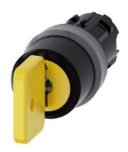
Key-operated switch O.M.R, 22 mm, round, plastic with metal front ring, lock number 73033, yellow, with 2 keys, 3 switch positions I-O-II, latching, actuating angle 2x45°, 10:30h/12h/13:30h, Key removal I+O+II, with laser labeling, lower case
