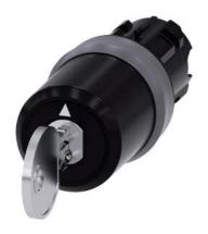
Key-operated switch BKS, 22 mm, round, plastic with metal front ring, lock No. E9 (VW), without key, 3 switch positions I-O-II, latching, actuating angle 2x45°, 10:30h/12h/13:30h, Key removal I+O+II, with laser labeling, upper case and lower case, always upper case at the beginning of the word
