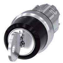
RONIS key-operated switch, 22 mm, round, metal, shiny, lock number SB30, with 2 keys, 3 switch positions I-O<II, left latching, right momentary contact type, actuating angle 2x45°, 10:30h/12h/13:30h, key removal O, possible special locks: SB31, 421, 455, with laser labeling, inscription or symbol Customer-specific selection with SIRIUS ACT configurator (CIN)
