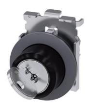
RONIS key-operated switch, 30 mm, round, Metal, matte, front ring for flush installation, lock number SB30, with 2 keys, 2 switch positions O-I, latching, actuating angle 90°, 10:30h/13:30h, key removal O+I, possible special locks: SB31, 421, 455, with laser labeling, upper case and lower case, always upper case at the beginning of the word
