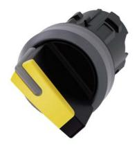
Selector switch, illuminable, 22 mm, round, plastic with metal front ring, yellow, selector switch, short, 2 switch positions O<I, momentary contact type, Actuating angle 45°, 10:30h/12h, with laser labeling, upper case and lower case, always upper case at the beginning of the word
