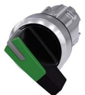
Selector switch, illuminable, 22 mm, round, metal, shiny, green, selector switch, long, 2 switch positions O-I, latching, actuating angle 90°, 10:30h/13:30h, Z=50-unit packaging
