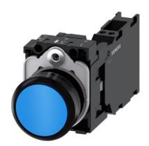
Pushbutton, 22 mm, round, plastic, blue, pushbutton, flat, momentary contact type, with holder 1 NO+1 NC, spring-type terminal, with laser labeling, upper case and lower case, always upper case at the beginning of the word
