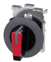
Selector switch, illuminable, 30 mm, round, Metal, matte, red, selector switch, short, front ring for flush installation, 3 switch positions I>O<II, momentary contact type, actuating angle 2x45°, 10:30h/12h/13:30h, with laser labeling, upper case and lower case, always upper case at the beginning of the word
