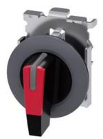
Selector switch, illuminable, 30 mm, round, Metal, matte, red, selector switch, long, front ring for flush installation, 3 switch positions I-O-II, latching, actuating angle 2x45°, 10:30h/12h/13:30h, with laser labeling, inscription or symbol Customer-specific selection with SIRIUS ACT configurator (CIN)
