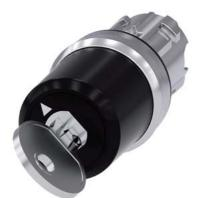
key-operated switch Siemens, 22 mm, round, metal, shiny, special lock, with 2 keys, 2 switch positions O-I, latching, actuating angle  $90^{\circ}$ , 10:30h/13:30h, key removal I
