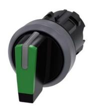
Selector switch, illuminable, 22 mm, round, plastic with metal front ring, green, selector switch, short, 3 switch positions I>O<II, momentary contact type, actuating angle 2x45°, 10:30h/12h/13:30h, with laser labeling, lower case
