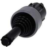
Coordinate switch, 22 mm, round, plastic with metal front ring, black, 2 switch positions, vertical, momentary contact type, with mechanical interlocking, with laser labeling, inscription or symbol Customer-specific selection with SIRIUS ACT configurator (CIN)
