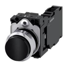
Pushbutton, 22 mm, round, metal, shiny, black, pushbutton, raised, momentary contact type, with holder, 1 NO+1 NC, screw terminal, with laser labeling, symbol number according to, ISO 7000 or IEC 60417
