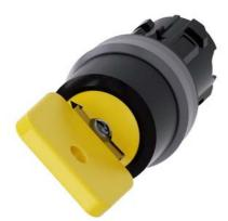
Key-operated switch O.M.R, 22 mm, round, plastic with metal front ring, lock number 73033, yellow, with 2 keys, 2 switch positions O-I, latching, actuating angle 90°, 10:30h/13:30h, key removal O, with laser labeling, lower case
