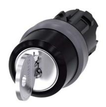
RONIS key-operated switch, 22 mm, round, plastic with metal front ring, lock number SB30, with 2 keys, 3 switch positions I-O<II, left latching, right momentary contact type, actuating angle 2x45°, 10:30h/12h/13:30h, key removal O+I, possible special locks: SB31, 421, 455, with laser labeling, upper case and lower case, always upper case at beginning of line
