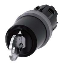
Key-operated switch IKON, 22 mm, round, plastic with metal front ring, lock number 360012K1, with 2 keys, 3 switch positions I-O-II, latching, actuating angle  $2x45^{\circ}$ , 10:30h/12h/13:30h, key removal O, with laser labeling, upper case and lower case, always upper case at beginning of line
