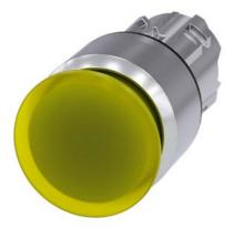
Illuminated mushroom pushbutton, 22 mm, round, metal, shiny, yellow, 30 mm, latching, pull-to-unlatch mechanism, with laser labeling, inscription or symbol Customer-specific selection with SIRIUS ACT configurator (CIN)
