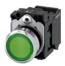
Illuminated pushbutton, 22 mm, round, Metal, shiny, green, pushbutton, flat, momentary contact type, with holder, 1NO, LED module with integrated LED 230 V AC, spring-type terminal, with laser labeling, upper case
