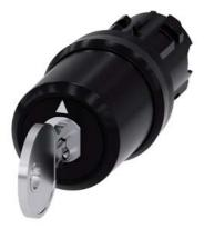
key-operated switch Siemens, 22 mm, round, plastic, special lock, with 2 keys, 3 switch positions I-O-II, latching, actuating angle  $2x45^\circ,\,10:30h/12h/13:30h,$  key removal I+O+II
