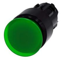
Illuminated mushroom pushbutton, 22 mm, round, plastic, green, 30 mm, latching, pull-to-unlatch mechanism, with laser labeling, lower case
