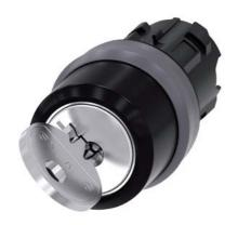
RONIS key-operated switch, 22 mm, round, plastic with metal front ring, lock number 455, with 2 keys, 2 switch positions O-I, latching, actuating angle  $90^\circ$ , 10:30h/13:30h, key removal O, with laser labeling, lower case
