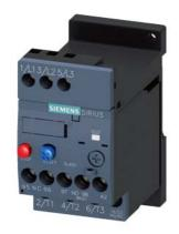
Overload relay 4.5...6.3 A Thermal For motor protection Size S00, Class 10 Stand-alone installation Main circuit: Screw Auxiliary circuit: Screw Manual-Automatic-Reset
