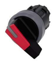
Selector switch, illuminable, 22 mm, round, plastic with metal front ring, red, selector switch, long, 2 switch positions O-I, latching, actuating angle  $90^\circ,\,10:30h/13:30h,\,Z=50-unit$  packaging
