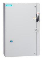
Non-reversing motor starter, Size 2 1/2, Three phase full voltage, Solid-state overload relay, OLR amp range 25-100A, 240V 50Hz / 277V 60Hz coil, Combination type, 100A fusible disconnect, 100A/250V fuse clip, Enclosure NEMA type 1, Indoor general purpose use, Extra-wide enclosure
