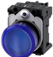
Indicator lights, 22 mm, round, plastic, blue, lens, smooth, with holder, LED module with integrated LED 110 V AC, screw terminal, with laser labeling, inscription or symbol Customer-specific selection with SIRIUS ACT configurator (CIN)
