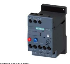
Overload relay 0.55...0.80 A Thermal For motor protection Size S00, Class 10 Stand-alone installation Main circuit: Screw Auxiliary circuit: Screw Manual-Automatic-Reset
