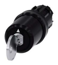
key-operated switch Siemens, 22 mm, round, plastic, lock number SSG10, with 2 keys, 3 switch positions I-O-II, latching, actuating angle 2x45°, 10:30h/12h/13:30h, key removal II, with laser labeling, upper case and lower case, always upper case at beginning of line
