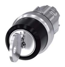
RONIS key-operated switch, 22 mm, round, metal, shiny, lock number SB30, with 2 keys, 3 switch positions I-O<II, left latching, right momentary contact type, actuating angle 2x45°, 10:30h/12h/13:30h, key removal I, possible special locks: SB31, 421, 455, with laser labeling, upper case and lower case, always upper case at beginning of line
