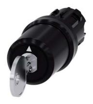
key-operated switch Siemens, 22 mm, round, plastic, lock number SSG10, with 2 keys, 3 switch positions I-O-II, latching, actuating angle 2x45°, 10:30h/12h/13:30h, key removal I, with laser labeling, upper case
