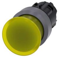
Illuminated mushroom pushbutton, 22 mm, round, plastic with metal front ring, yellow, 30 mm, momentary contact type, with laser labeling, lower case
