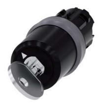
key-operated switch Siemens, 22 mm, round, plastic with metal front ring, lock number SSG10, with 2 keys, 2 switch positions O-I, latching, actuating angle 90°, 10:30h/13:30h, key removal O, with laser labeling, lower case
