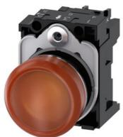
Indicator lights, 22 mm, round, metal, shiny, amber, lens, smooth, with holder, LED module with integrated LED 24 V AC/DC, screw terminal, with laser labeling, symbol number according to, ISO 7000 or IEC 60417
