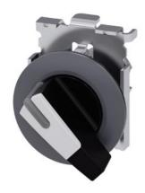
Selector switch, illuminable, 30 mm, round, Metal, matte, white, selector switch, long, front ring for flush installation, 2 switch positions O-I, latching, actuating angle  $90^\circ,\,10:\!30h/13:\!30h,$  with laser labeling, upper case and lower case, always upper case at the beginning of the word
