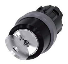
RONIS key-operated switch, 22 mm, round, plastic with metal front ring, lock number 455, with 2 keys, 2 switch positions O-I, latching, actuating angle 90°, 10:30h/13:30h, key removal O+I, with laser labeling, lower case
