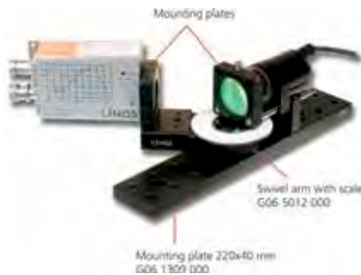
Application example of Swivel arm with scale
