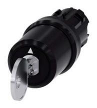
key-operated switch Siemens, 22 mm, round, plastic, lock number SSG10, with 2 keys, 3 switch positions I-O-II, latching, actuating angle 2x45°, 10:30h/12h/13:30h, key removal II, with laser labeling, inscription or symbol customer-specific selection with SIRIUS ACT configurator (CIN)
