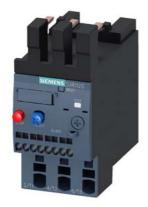
Overload relay 7.0...10 A Thermal For motor protection Size S0, Class 10 Contactor mounting Main circuit: Spring-type terminal Auxiliary circuit: spring-type terminal Manual-Automatic-Reset
