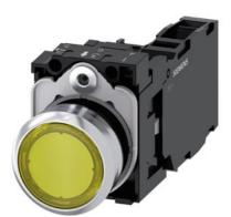
Illuminated pushbutton, 22 mm, round, metal, shiny, yellow, pushbutton, flat, momentary contact type, with holder, 1 NO+1 NC, LED module with integrated LED 110 V AC, screw terminal, with laser labeling, symbol number according to, ISO 7000 or IEC 60417
