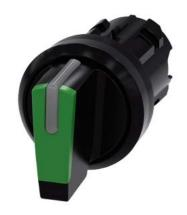
Selector switch, illuminable, 22 mm, round, plastic, green, selector switch, short, 3 switch positions I>O<II, momentary contact type, actuating angle 2x45°, 10:30h/12h/13:30h, with laser labeling, upper case and lower case, always upper case at the beginning of the word
