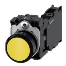
Pushbutton, 22 mm, round, plastic, yellow, pushbutton, flat, momentary contact type, with holder 1 NO+1 NC, spring-type terminal, with laser labeling, upper case and lower case, always upper case at beginning of line
