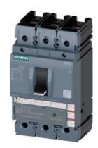
circuit breaker 3VA5 UL frame 250 breaking capacity class H 65kA @ 480 V 3-pole, line protection TM230, FTAM, In=110A overload protection Ir=110A fixed short-circuit protection Ii=5...10 x In UL489 SB (naval), 50 deg. cel. nut keeper kit on both sides
