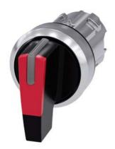
Selector switch, illuminable, 22 mm, round, metal, shiny, red, selector switch, long, 3 switch positions I-O<II, left latching, right momentary contact type, actuating angle  $2x45^{\circ}$ , 10:30h/12h/13:30h, Z=50-unit packaging
