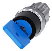
Key-operated switch O.M.R, 22 mm, round, metal, shiny, lock number 73038, blue, with 2 keys, 2 switch positions O-I, latching, actuating angle  $90^{\circ}$ , 10:30h/13:30h, key removal O+I, Z=50-unit packaging
