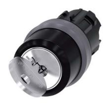
RONIS key-operated switch, 22 mm, round, plastic with metal front ring, lock number 455, with 2 keys, 2 switch positions O-I, latching, actuating angle  $90^\circ$ , 10:30h/13:30h, key removal O, with laser labeling, upper case
