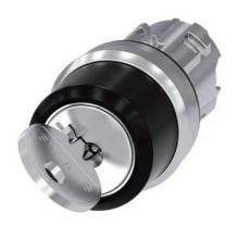
RONIS key-operated switch, 22 mm, round, metal, shiny, lock number 455, with 2 keys, 2 switch positions O<I, momentary contact type, Actuating angle 45°, 10:30h/12h, key removal O, with laser labeling, upper case and lower case, always upper case at the beginning of the word
