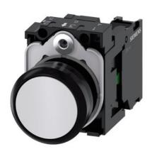
Pushbutton, 22 mm, round, plastic, white, pushbutton, flat, momentary contact type, with holder 1 NO, screw terminal, with laser labeling, inscription or symbol Customer-specific selection with SIRIUS ACT configurator (CIN)
