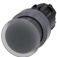
Illuminated mushroom pushbutton, 22 mm, round, plastic with metal front ring, clear, 30 mm, momentary contact type, with laser labeling, lower case
