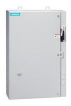
Non-reversing motor starter, Size 1, Three phase full voltage, Solid-state overload relay, OLR amp range 10-40A, Combination type, 60A fusible disconnect, 60A/250V fuse clip, Enclosure NEMA type 4/12, Water/dust tight for outdoors, Extra-wide enclosure
