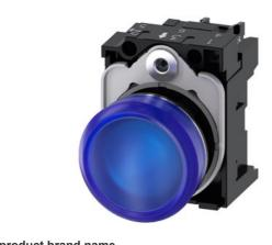
Indicator lights, 22 mm, round, Metal, shiny, blue, lens, smooth, with holder, LED module with integrated LED 230 V AC, screw terminal, with laser labeling, upper case and lower case, always upper case at the beginning of the word
