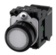
Illuminated pushbutton, 22 mm, round, plastic, clear, pushbutton, flat, momentary contact type, with holder, 1NO, LED module with integrated LED 230 V AC, spring-type terminal, Z=20-unit packaging
